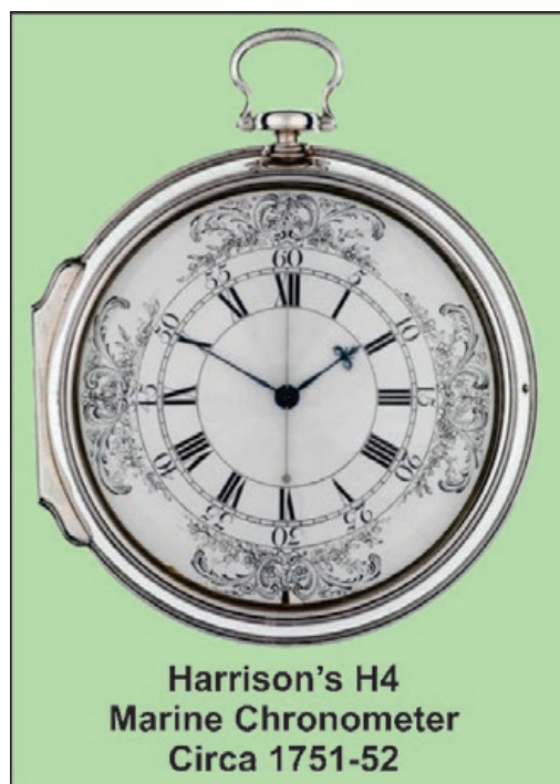
Figure 1. James Harrison's H4 Chronometer allowed longitude determination.
